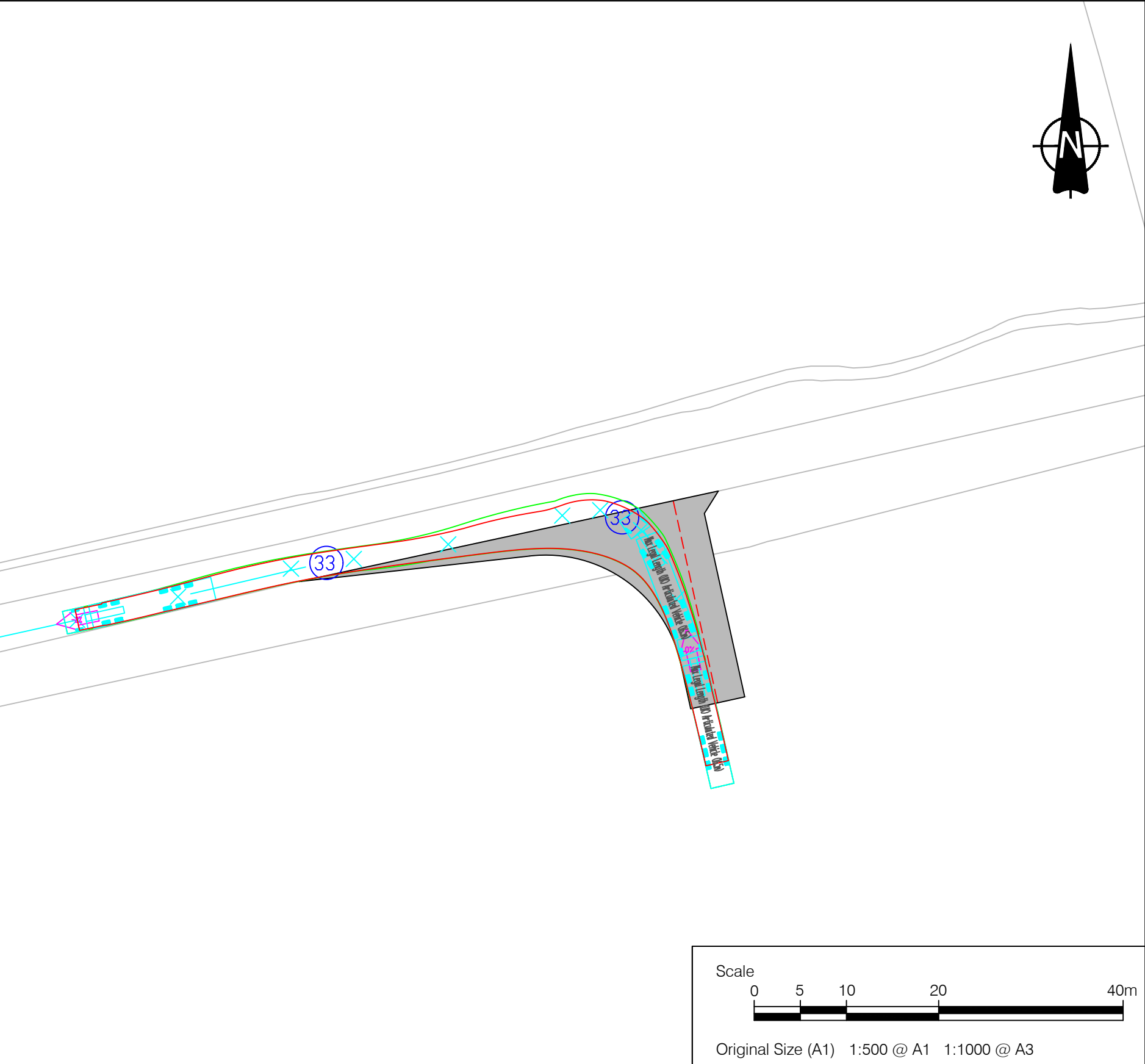
INSET B: HGV MANOEUVRE HEADING OUT OF ACCESS, LEFT TURN ONTO MOOR LANE HEADING WEST - SCALE 1:500
